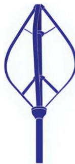
Figure 6: Darrieus blade design.
