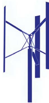
Figure 9: H-Rotor blade design.
